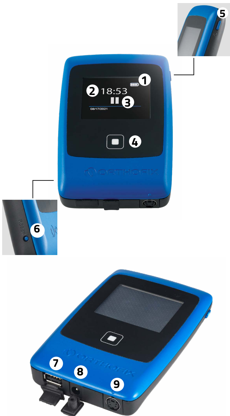
Figure 3 : The AccelStim device Generator
