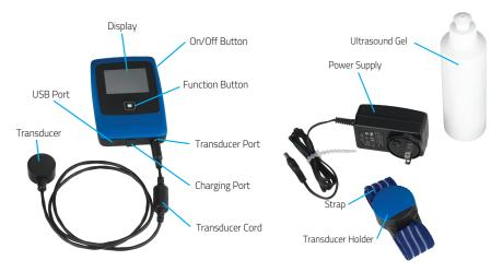
Figure 2: AccelStim device components
